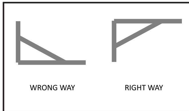
placing the horizontal beam at the top will allow this to represent an extension of the roof beam, to be high enough above the loading platform to support a pulley, and to put the diagonal member in compression, as it needs to be, since wood is weak in tension. Fortunately, the mounting boss is centered, so no modification is needed to orient the part correctly.
